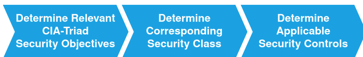
Figure-A-2: High level security requirements identification process.
